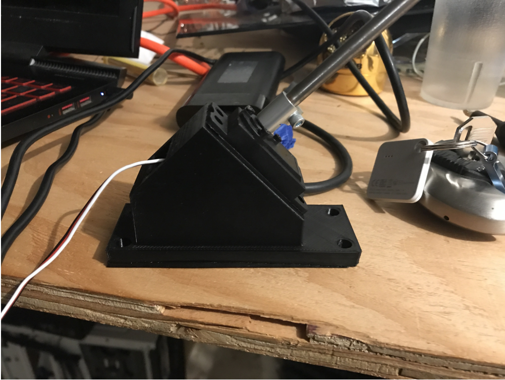
Fig. 3.16. Second Iteration of Propulsion System Bracket Holding Propulsion System
