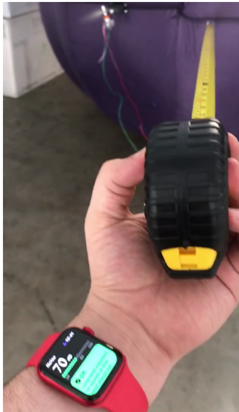
Fig. 9.2. Noise Test Being Conducted.
