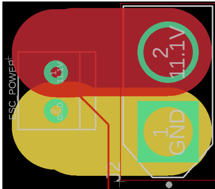
Fig. 5.24. Trace Between 12V Battery Pinout (right) to ESC Pinout (left)
