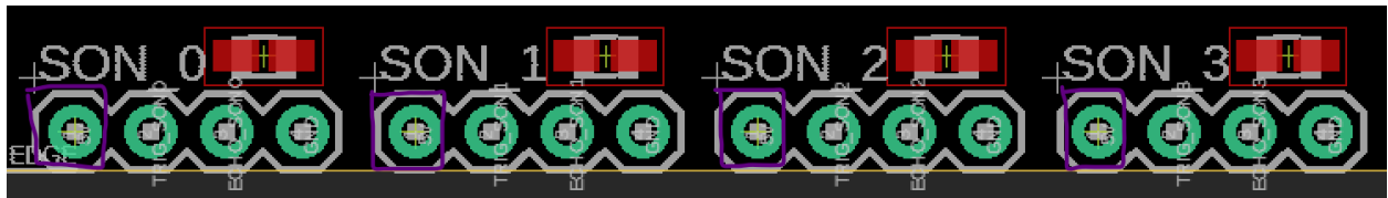
Fig. 5.40. Ultrasonic Sensor 5V Test Points (Boxed in Purple)
